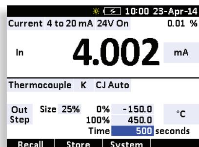
Set up span, step size and timing, step and ramp times up to 999 seconds.
